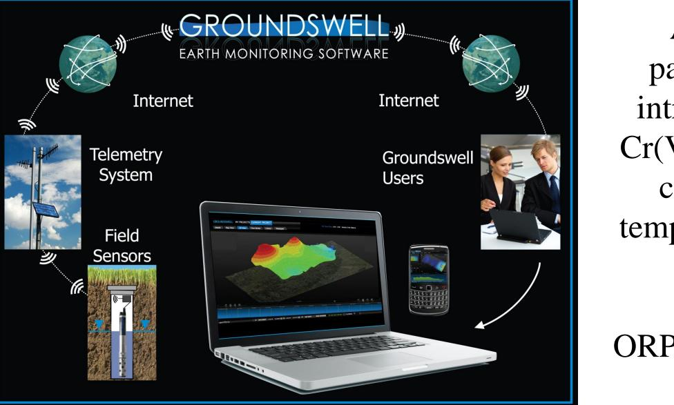
Automated monitoring parameters include: vapor intrusion VOCs,  $CH_4$ , TCE, Cr(VI),  $CCl_4$ , nitrate, atrazine, chlorophyll, water level, temperature, pH, conductivity, salinity, Br<sup>-</sup>,  $Cl^{-}, NH_{4}^{+}, DO,$ ORP, oceanographic attributes.
