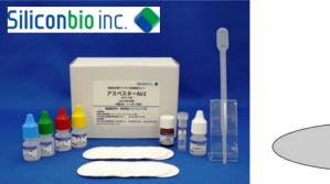
In collaboration with Hiroshima University, Siliconbio® has developed an airborne asbestos detection kit (Asbester **AIR**), using a fluorescently labeled DksA or GatZ protein probes that selectively bind to asbestos fibers. Following airborne dust sampling, just a few drops of reagents are applied onto a membrane filter. Immediate sample observation and high contrast imaging are possible without any complicated sample preparation.
