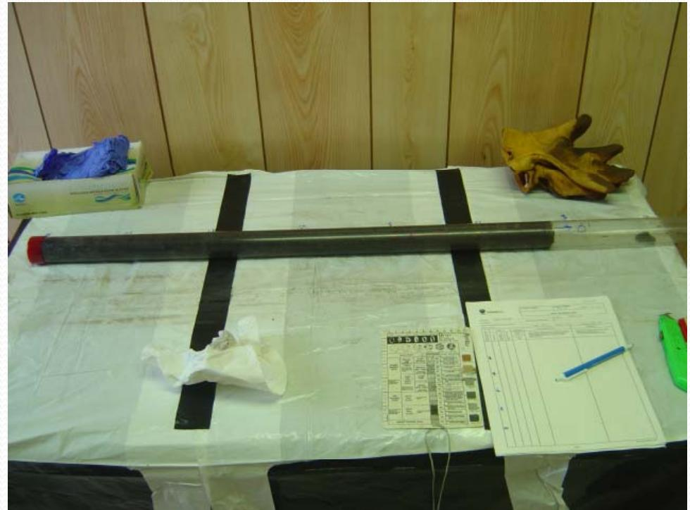
Core obtained from the field before freezing
