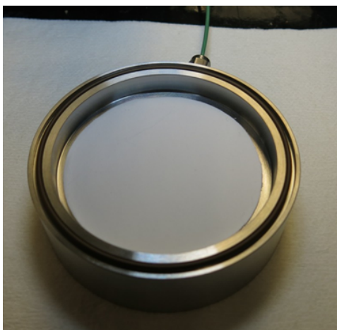
Internal 58mm internal glass-fiber filter with 1-(2-pyridyl)piperazine (PP)
