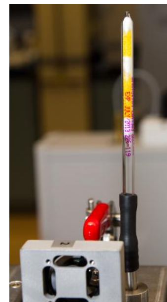
Silica gel with DNPH tube
