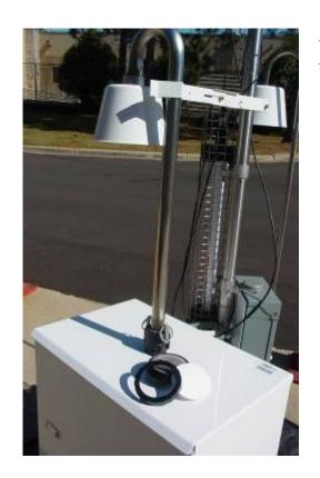
Deployable air monitors utilize a glass 4"filter and a glass 2" filter. Alternatively, 2" silver zeolite or charcoal cartridges may be substituted for sampling select nuclides.
