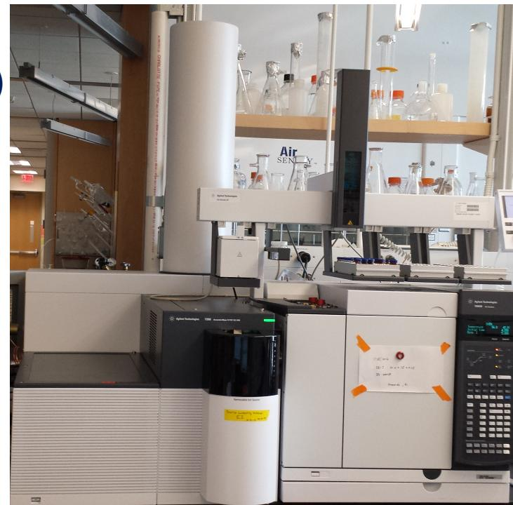
Figure. Shown above is the Agilent 7200 GC/Q-TOF. It is equipped with the PAL autosampler.
