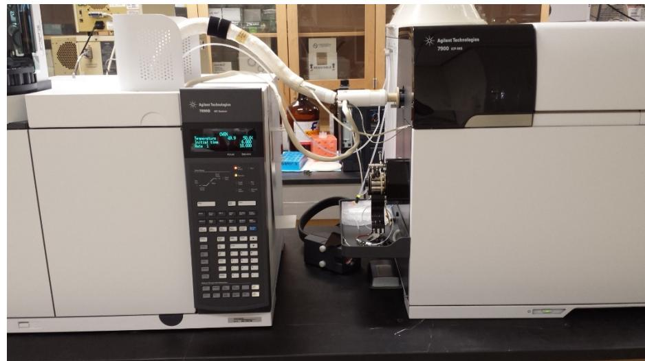
Figure. Shown above is the Agilent 7890B/ 7900 GC-ICPMS.
