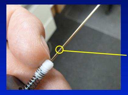
Side Hole -vacuum applied here during sampling -serves as carrier gas inlet during desorption
