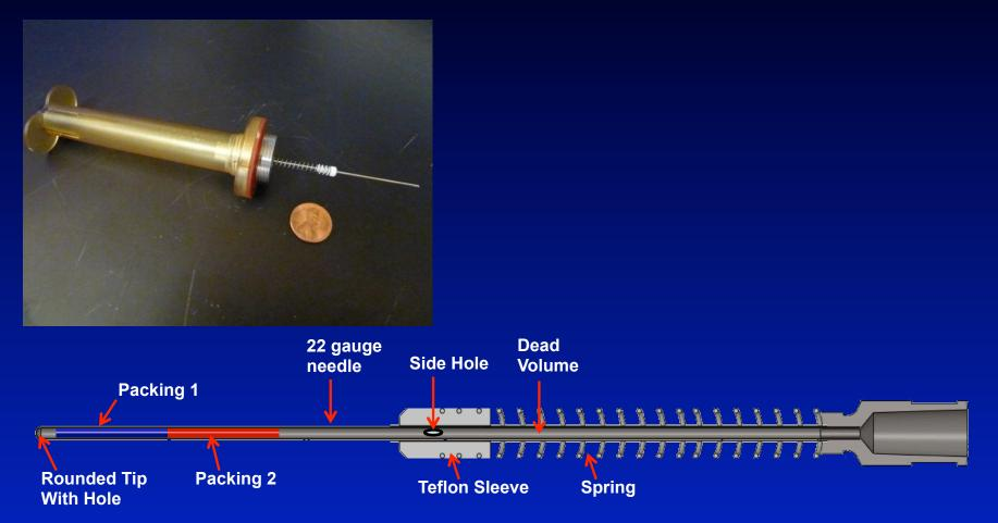
Several milligrams of different sorbents with increasing strength packed in small needle (similar to large tubes except for scale)
