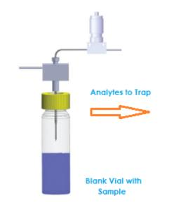
The sample is heated and purged in the same manner as a soil sample, and the analytes are trapped on the analytical trap. Next, the analytes are desorbed onto the GC column.
