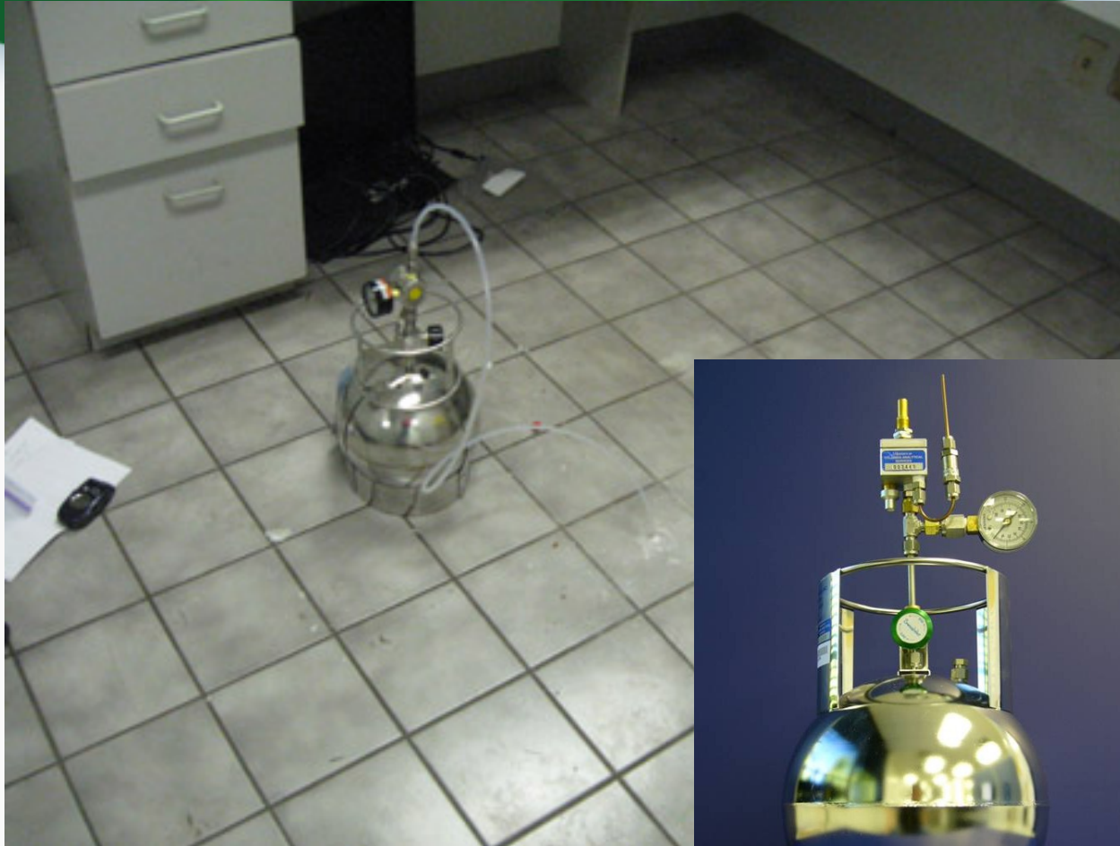
Residential SS sampling using sampling probe and SUMMA canister
