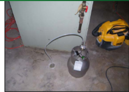
Residential SS sampling using sampling probe and SUMMA canister
