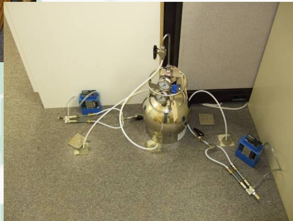
TO-15 and TO-17 sample methods side by side
