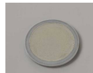
Sample Appearance (Press-formed at 250 kN for 30 sec)
