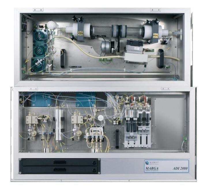
Photo of MARGA instrument (Metrohm Applikon, the Netherlands). The sampling compartment (top) contains the Wet Rotating Denuder (WRD) that removes and samples soluble gases (HNO<sub>3</sub>, HONO, SO<sub>2</sub>) from a sampled airflow prior to entry into the Steam Jet Aerosol Collector (SJAC) where soluble particles are grown by deliquescence, removed, and sampled via impaction. Samples are then fed semicontinuously on the hour into an on-line ion chromatography analyzer.
