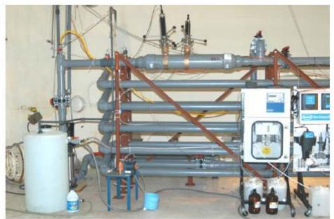
Figure 4: Hach HST constructed a special variable volume flow loop inside of an ECBC surety chamber.
