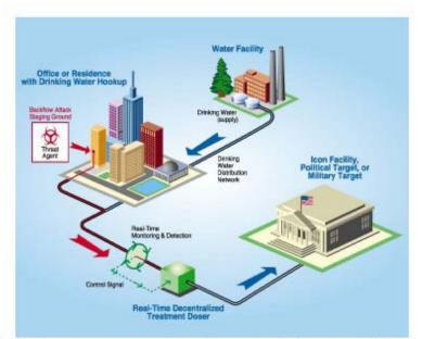
Figure 2: All distribution systems are vulnerable to a backflow attack. The attack point can be anywhere in the system.
