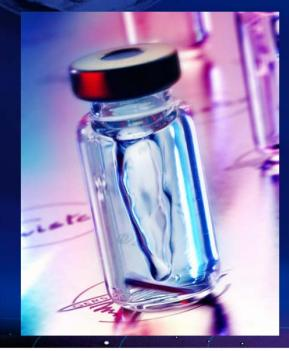
A PDMS-coated stir bar (GERSTEL Twister) is added to the vial
