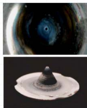
Cones after SC-Fast 740 analysis
