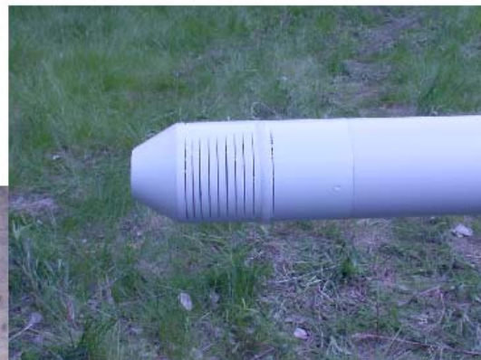
EPA Installed 12 2-inch PVC monitoring wells with 2-inch screened interval using Geoprobe direct push technique
