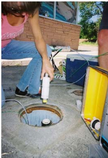
Inserting PDS and messenger into 2-inch monitoring well
