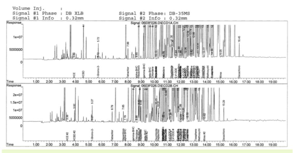
• Laboratory reported only 3 of 32 OC pesticides as detected: gamma-Chlordane at 190 *PD* ug/kg, Endrin at 5.7 *P* ug/kg, and 2,4′-DDD at 250 *D*, ug/kg (analysis at 1x and 50x dil.). Analysis by HRGC/MS/MS reported 9 of 31 OC pesticides as detected. A1260 reported at 6,500 ug/Kg in this sample
