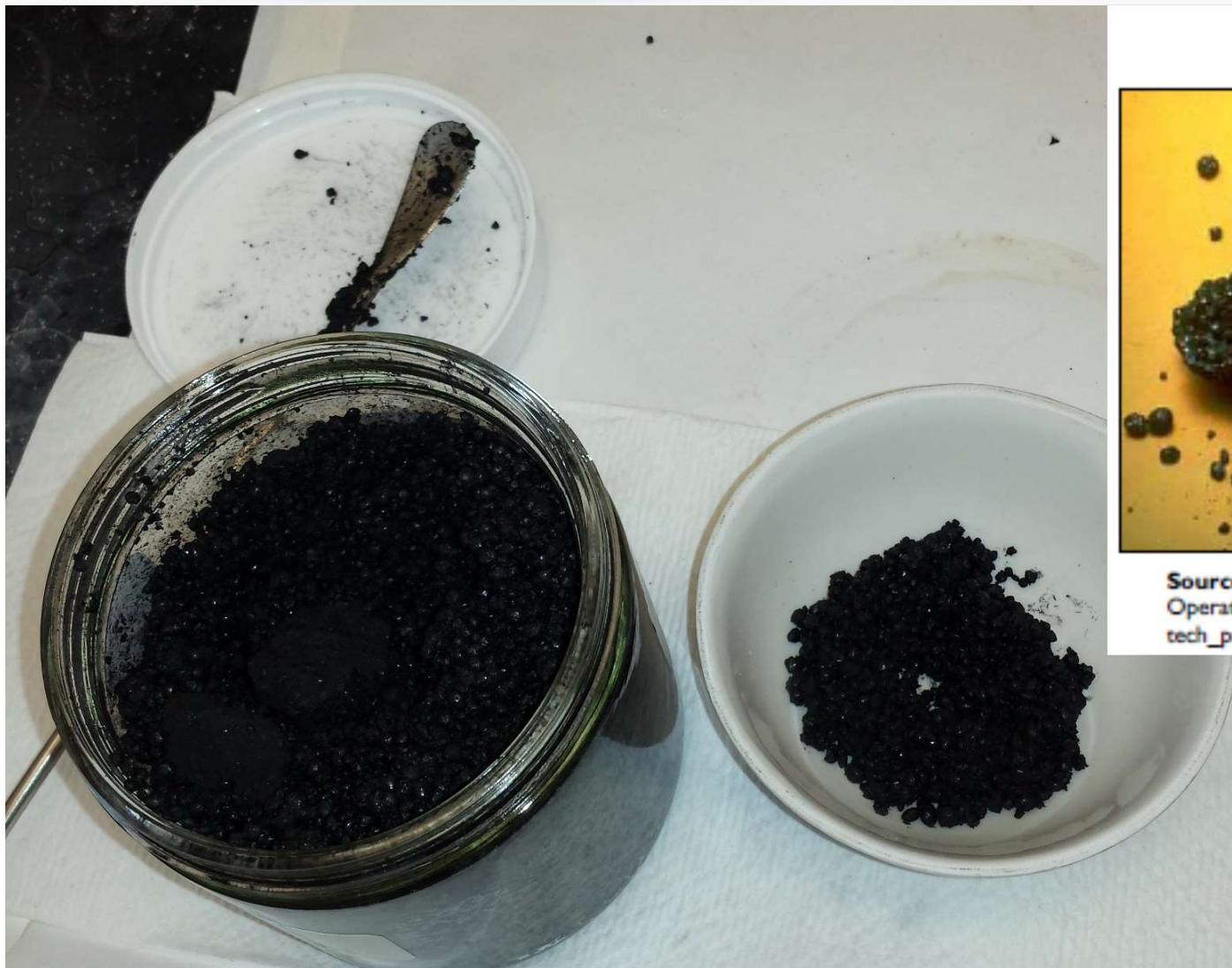
Figure 2. Shot Coke Partially Crushed
