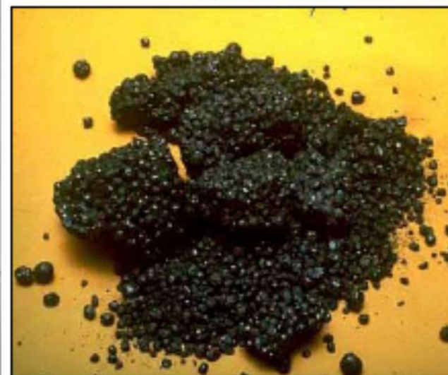
Figure 2. Shot Coke Partially Crushed
