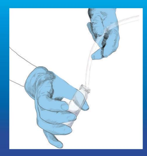
Direct Fill – A VOA vial is filled directly from the tap or tubing, using a low flow to prevent aeration or turbulence.
