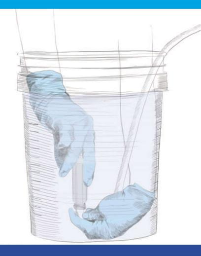
Inverted Fill – A VOA vial is inverted in a bucket of purge water and filled by displacement.
