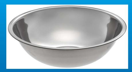
Bowl Method – A shallow bowl is filled with water, and the VOA vial is dipped in to fill.
