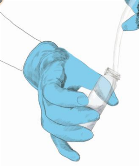
Open System Direct Fill Method (40 ml VOA vials)
