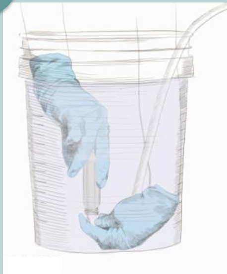
"Semi-closed" System Inverted Bottle Method (40 ml VOA vials)
