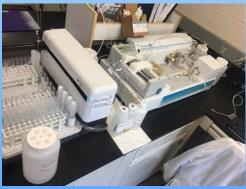
OI Analytical FS3700 Segmented Flow Analyzer, Set Up for TKN by EPA 351.2
