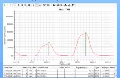
TKN determination using peak height takes 2 minutes per sample vs. approximately 6-8 minutes for distillation and titration using method SM-4500 NH3, Kjeldahl Nitrogen.
