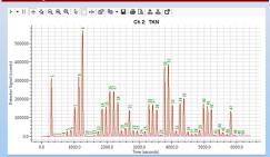
The graph above shows a Kjeldahl run by method EPA 351.2 consisting of calibration standards, quality control samples, matrix spikes, and 24 unknown samples with a total time of approximately 103 minutes.
