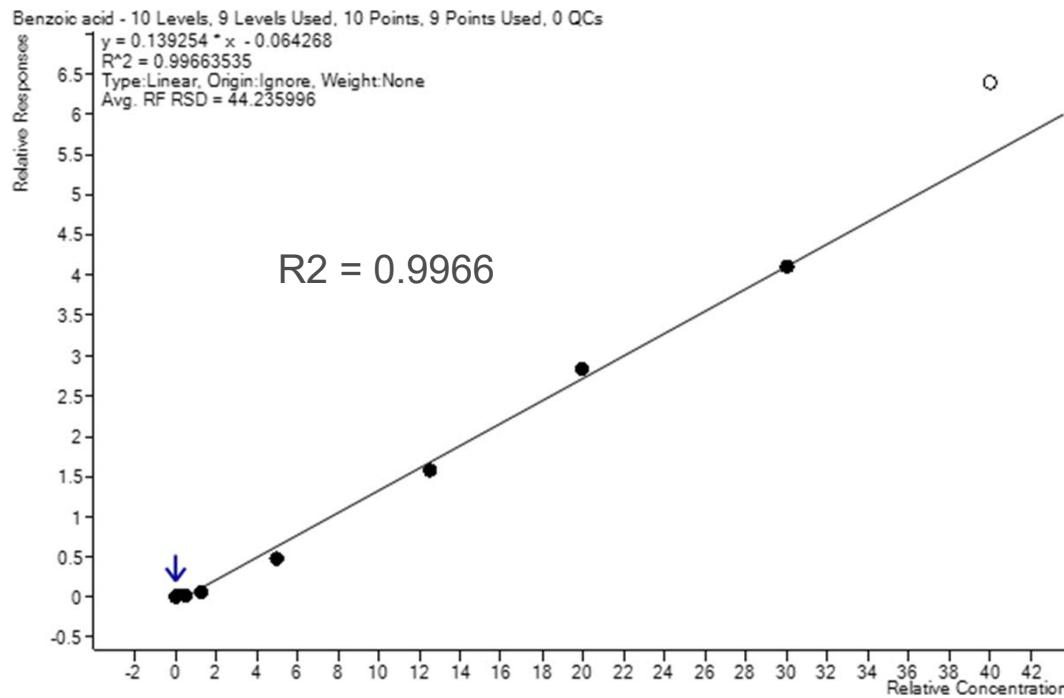
Calibration results for the challenging compound benzoic acid (0.05 – 120 ppm)
