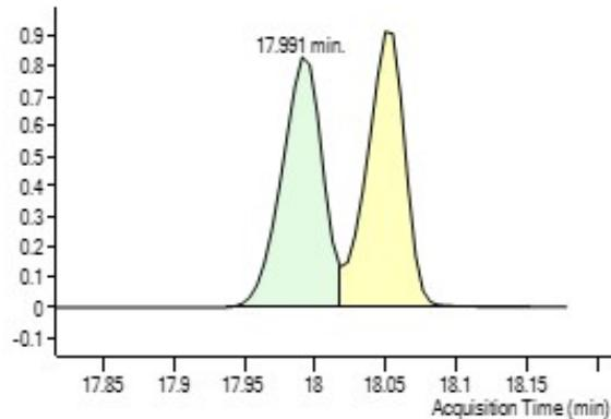
50 ppm, 1:3 split, LPD liner, 9 mm lens (17 ng injected)
