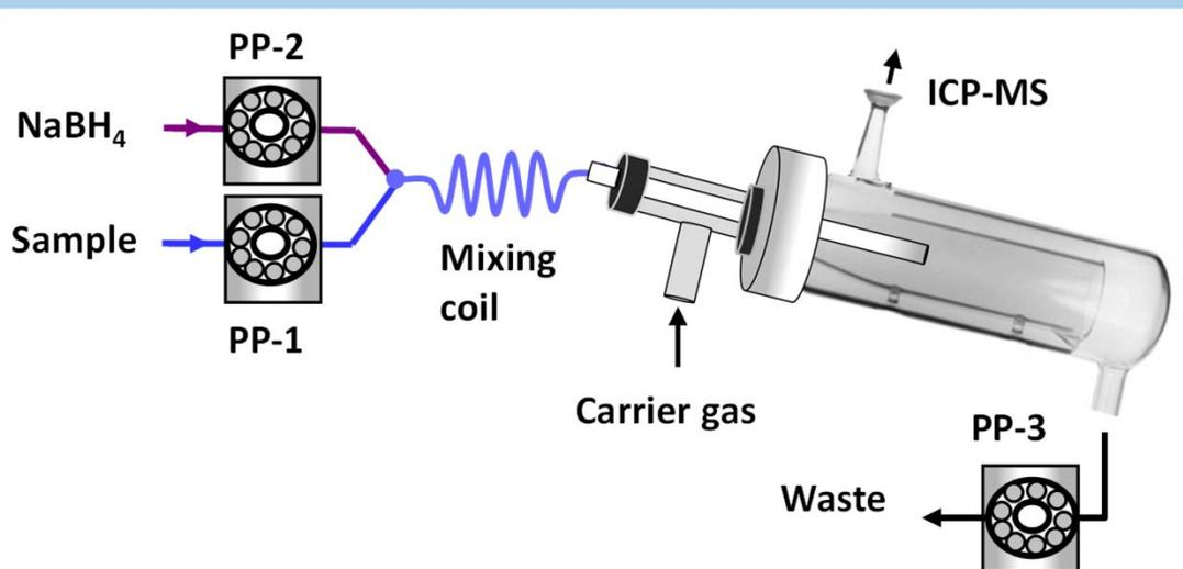
Cold vapor generation manifold and ICP-MS instrument for determination of  $\text{CH}_3\text{Hg}$
