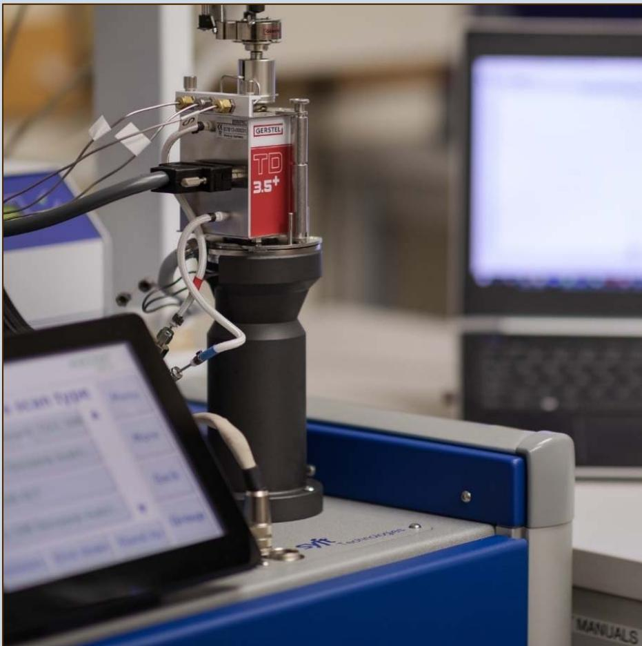
Utilizes GERSTEL TD 3.5<sup>+</sup> for analysis of standard 3.5" tubes
