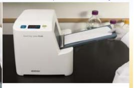
Seal using the Quanti-Tray Sealer PLUS and incubate for 7 days.
